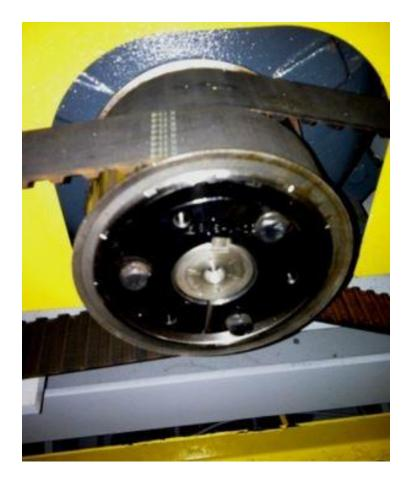
**Gearbelt Pulley & Bushing**
