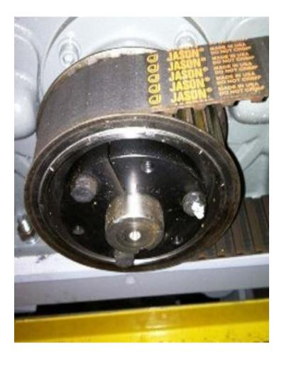
**Gearbelt Pulley & Bushing**
